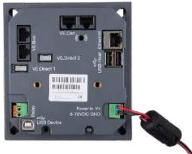
Connect the LAN1 port of the Elum Explorer to the Ethernet port of the Victron Color Control.
