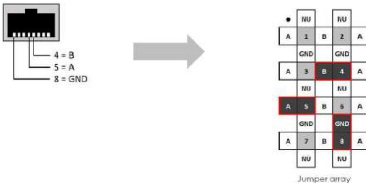
Figure 2: Pin mapping jumper array
