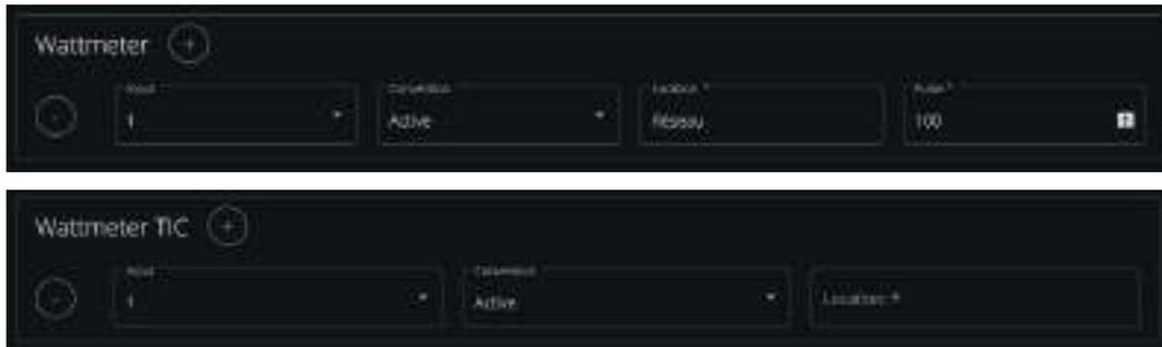
The “Active” Convention must be applied on the meters that are measuring production. The “Passive” convention must be set for meters measuring consumption.
